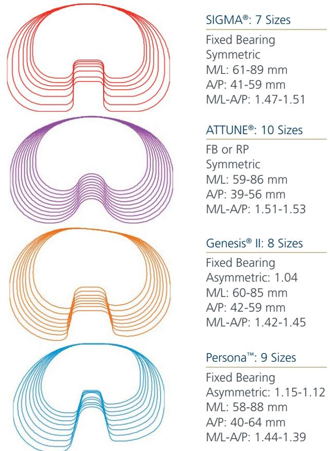
Figure 1: Tibial base designs analyzed in this study
