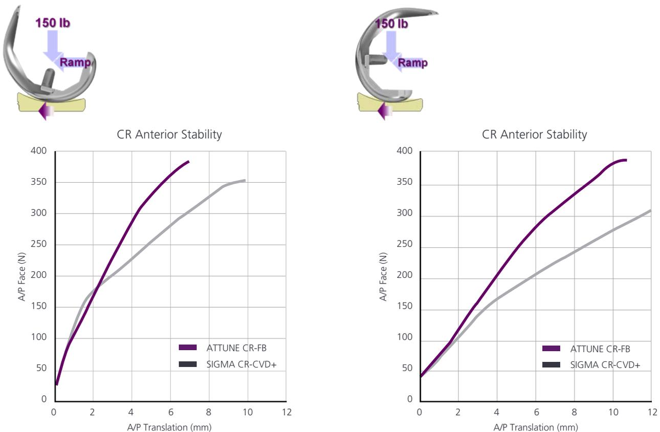
Figure 5: A/P stability of CS fixed bearing designs (ATTUNE CR and SIGMA CVD+) at 15 and 90 degrees of flexion.
