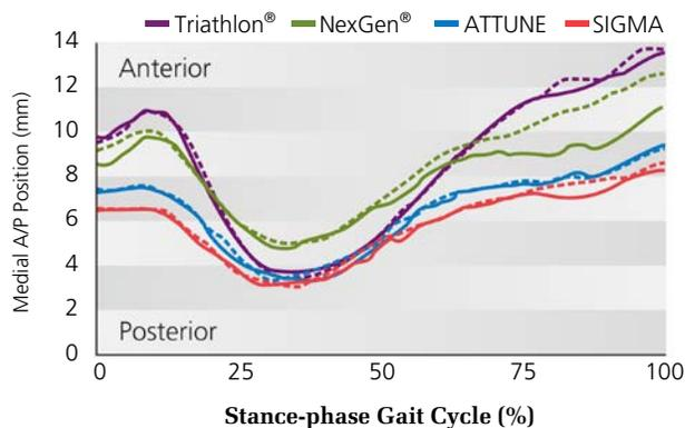
Figure 7: This graph shows the A/P movement of Triathlon®, NexGen®, the ATTUNE Knee, and SIGMA Curved throughout the stance phase of gait. Note: The more vertical variation in a line, the greater the A/P movement
