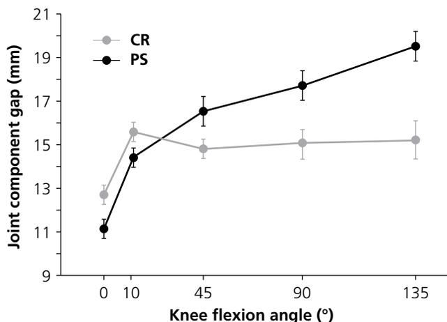
Figure 3: Graph showing the flexion space opening up in a PS knee versus a CR knee as the knee flexes
