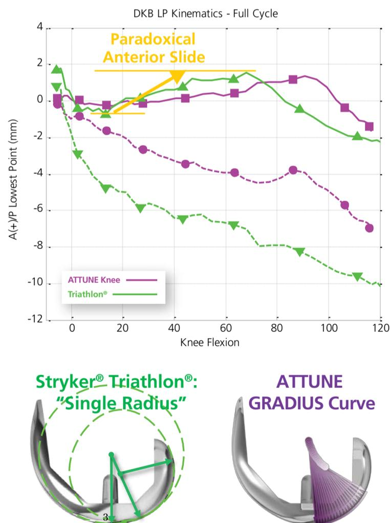
Figure 4: The results from the cadaveric testing at the University of Kansas clearly demonstrates the paradoxical anterior slide which occurs at the transition from the distal to posterior radii in traditional knee replacement. The anterior slide was significantly reduced in the cadaveric knees implanted with the ATTUNE Knee.
