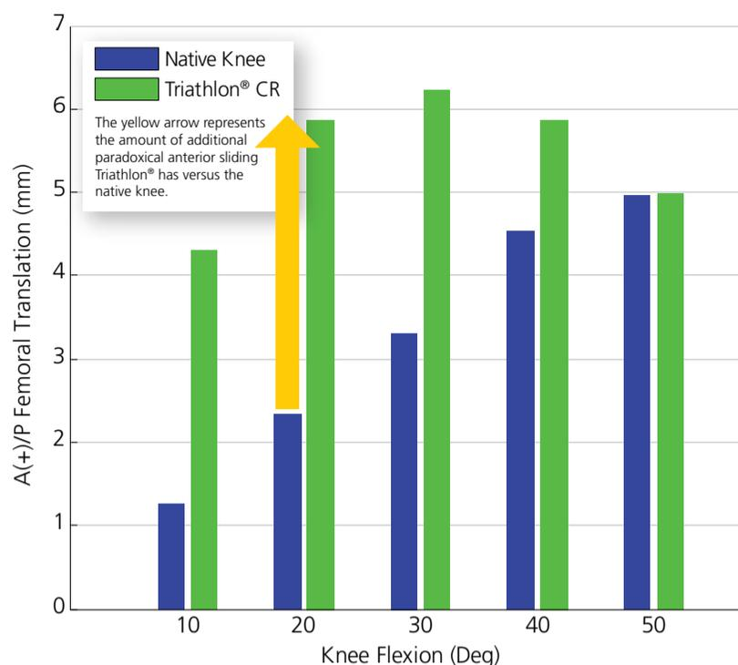
Figure 3: The overall A/P range of motion for the native knee and the Triathlon® total knee reported by Stoddard et al, demonstrating that the Triathlon® has significantly less constraint in knee extension and mid flexion.<sup>7</sup>
