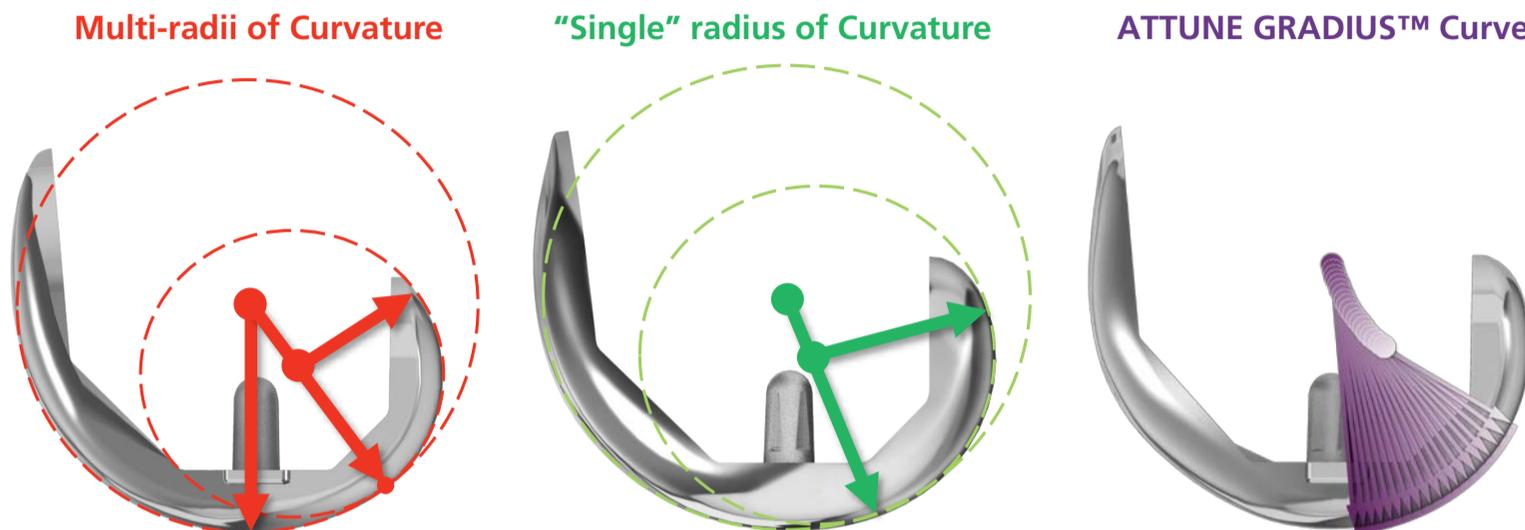
Figure 1: The sagittal plane curvature of “traditional” knee replacements are comprised of multiple discrete radii. While the Stryker® Triathlon® is formed by a single radius of flexion, the ATTUNE Knee incorporates a gradually reducing radius with knee flexion (ATTUNE GRADIUS Curve)
