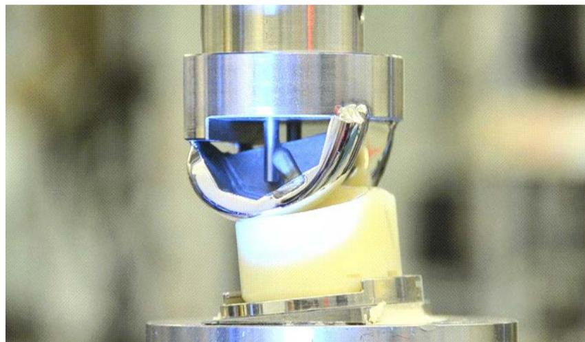
Figure 4 – Schematic of Anterior Tab Testing During Posterior Tibio-Femoral Translation
