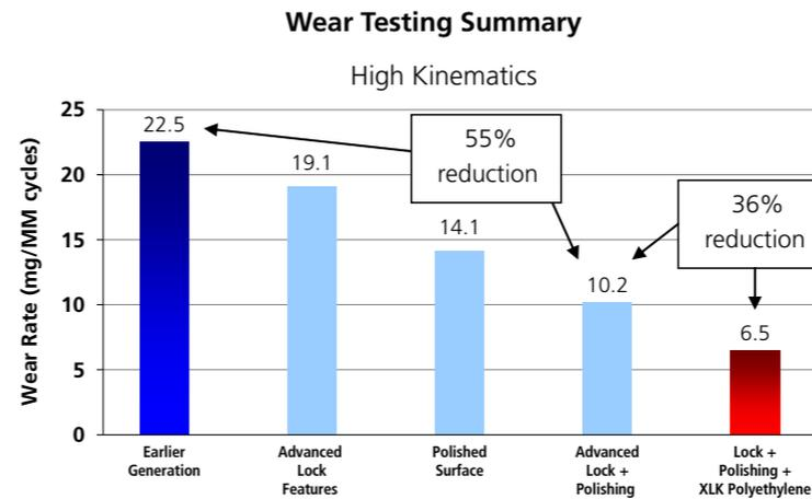
Figure 6 – Relative Effects of Design Features Upon Total Polyethylene Wear<sup>14</sup>
