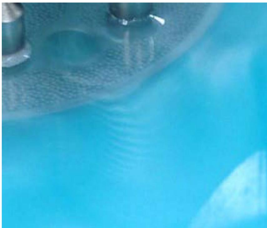
**Competitive tibial base plate demonstrating fluid flow exiting distal fixation screw holes**
