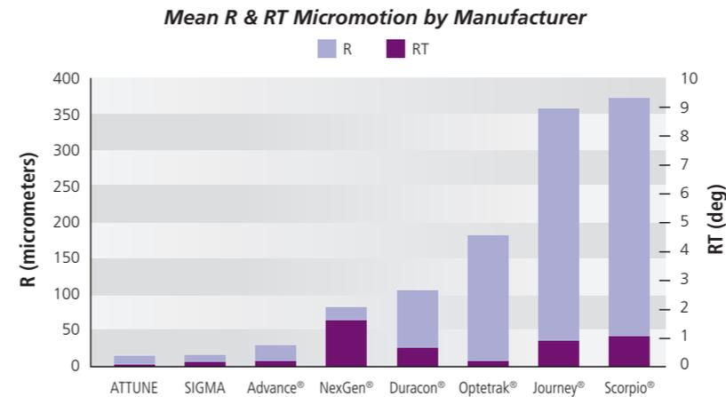
R – Vector summation of A/P & M/L micromotion, RT – Torsion micromotion due to I/E rotation
