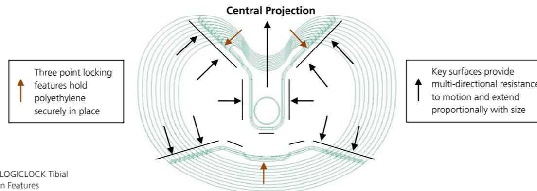
Figure 3 – LOGICLOCK Tibial Base Design Features
