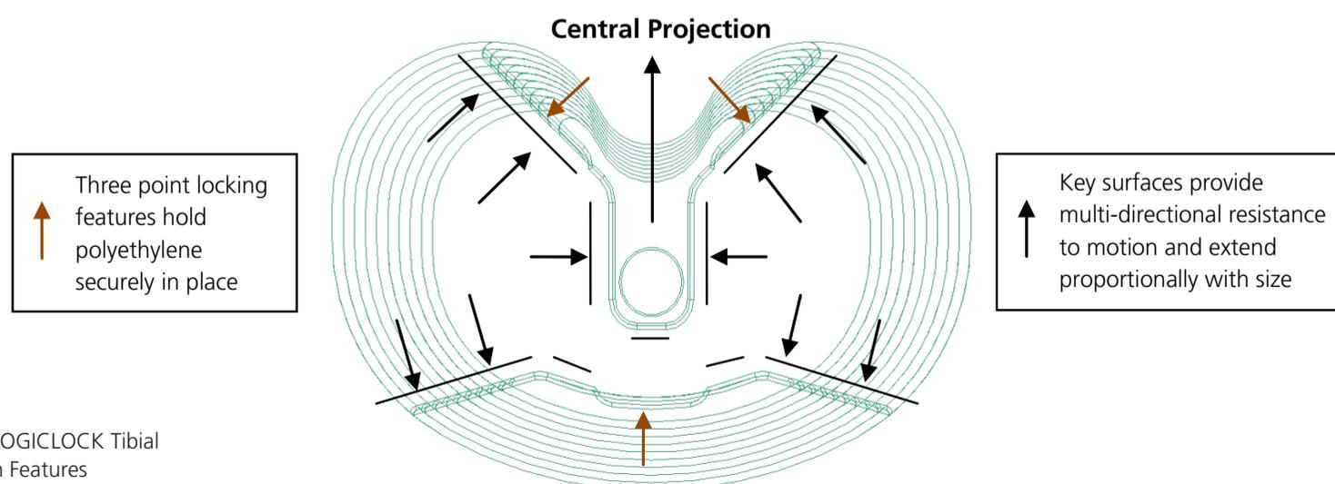
Figure 3 – LOGICLOCK Tibial Base Design Features
