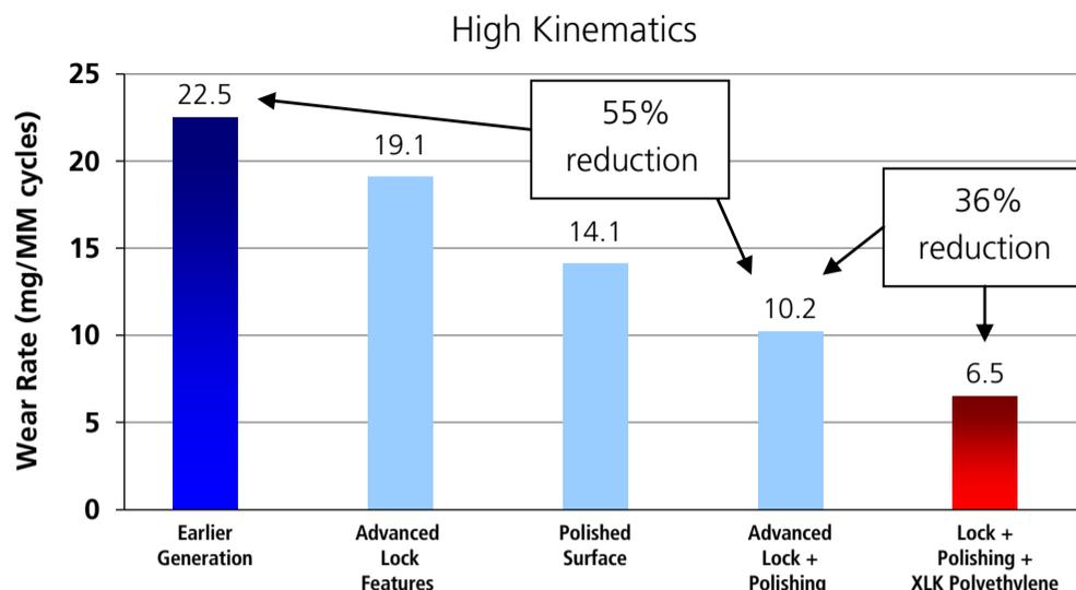
Figure 6 – Relative Effects of Design Features Upon Total Polyethylene Wear<sup>14</sup>
