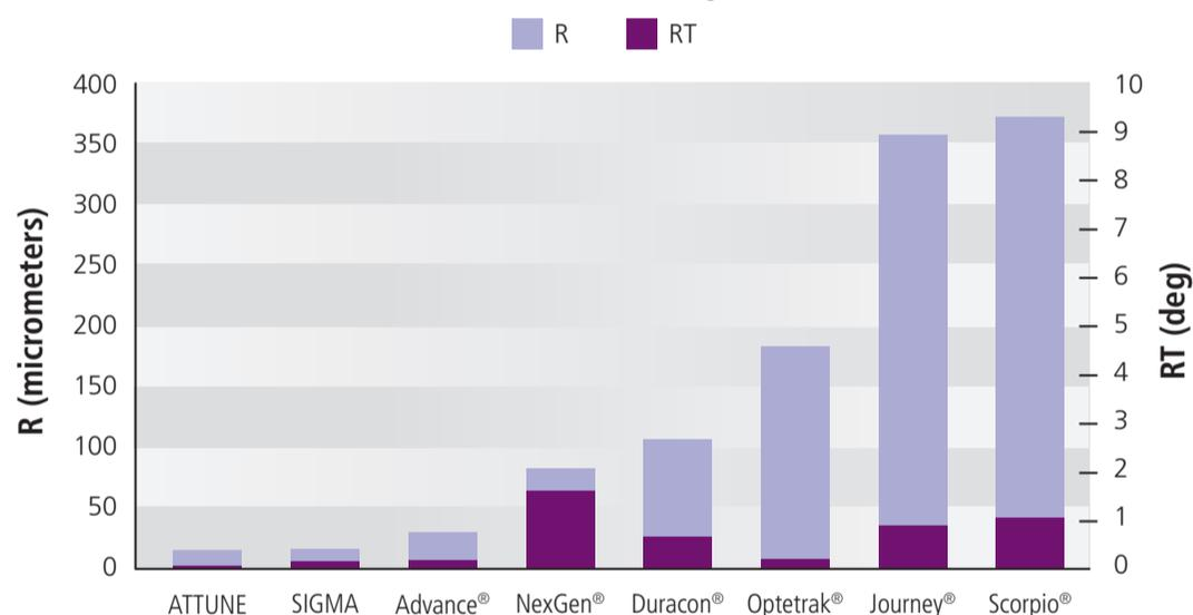
R – Vector summation of A/P & M/L micromotion, RT – Torsion micromotion due to I/E rotation
